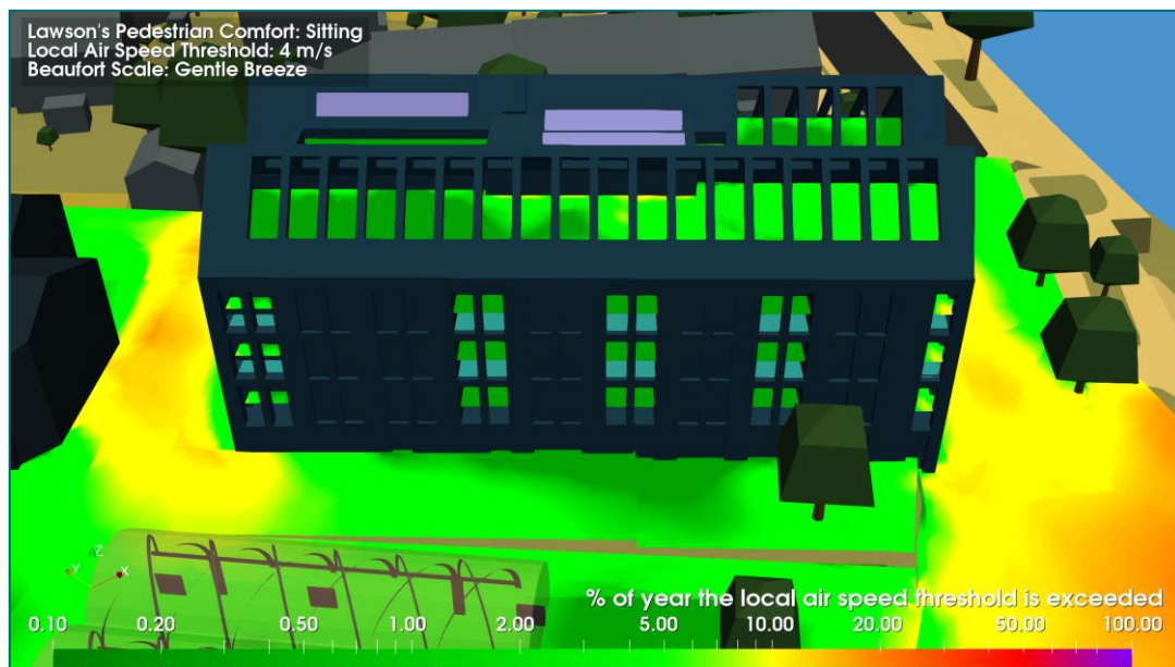
Figure 26: Sitting Comfort Criterion: OCS Block: Balconies: View from the southwest
